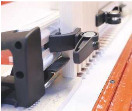
▲ Work locates against a side stop
